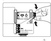
Adjust the gain knob as needed while recording. You can check the gain level on the left side of the knob.
