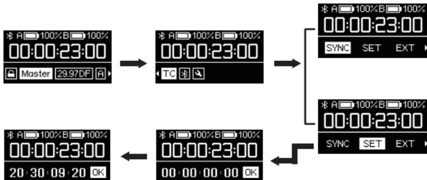
Note: During Master Run mode, TC-SL1 also can be jam-synced by an external timecode source or other TC-1 via the 5P cable. Set TC-SL1 mode to Master Run mode, enter TC setting, select EXT option and TC-SL1 will detect the external timecode and frame rate automatically. Press the function control wheel to select Jam and synchronize to an external timecode source.
