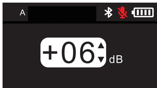
Long press the “Down direction key” to enter the output gain adjustment mode of the output port B. You can adjust the output gain through the “Up/Down” direction key. There are 31 gears of gain adjustment, and the gain can be customized according to the usage scene. The adjustable output range is -20 ~ +10dB.
