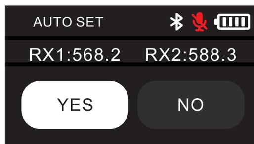
Click "YES" to send the synchronously scanned frequency points to the transmitter, and click "NO" to cancel the synchronous frequency point distribution.
